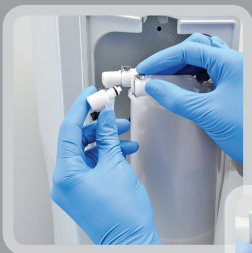
Quick-connect cartridge replacement
