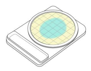
Specimen diffuses automatically and evenly into all over the sheet (total medium of 20 cm2) to transform it into gel within seconds.
